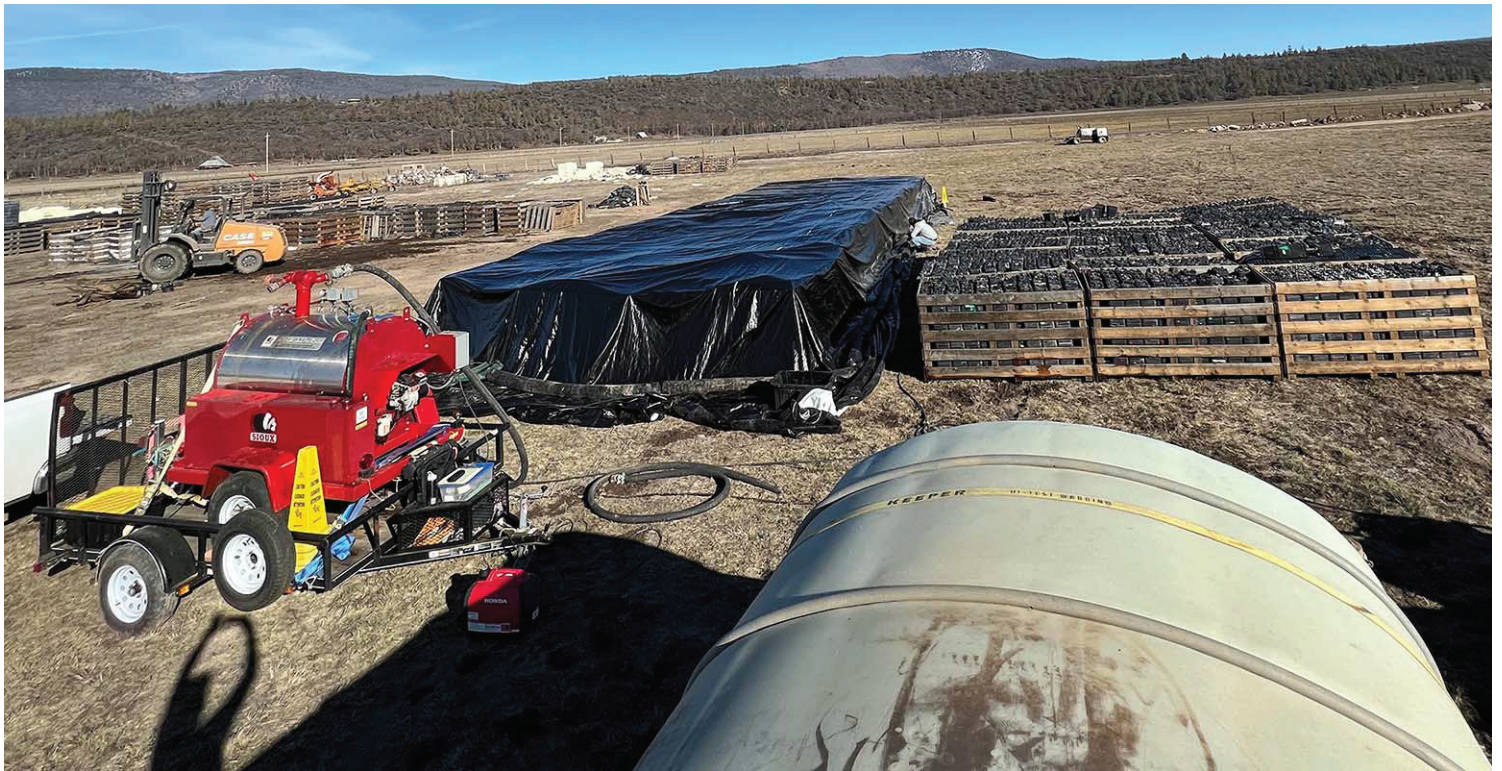
Figure 3. ‘Steaming-on-the-Go’ of huge numbers of pots can be achieved in a relatively short time at low costs.
